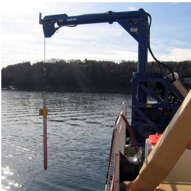
FFCPT integrated with an MVP200 on CCGS Matthew.
