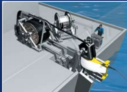
Launch, tow and recovery system for active and passive sonar
