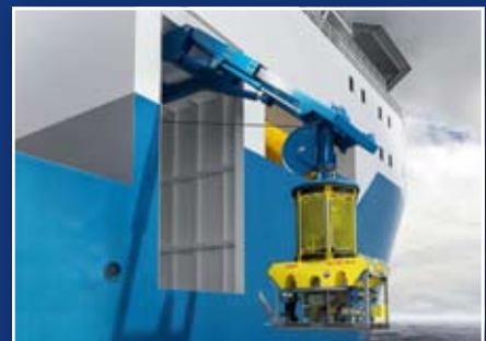
Deckhead-mounted handling equipment for mission bays
