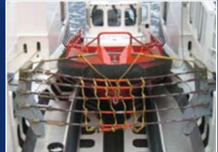
Stern ramp for work boats and USVs
